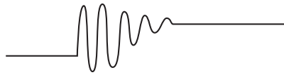
The signal oscillates between states after a mechanical switch or relay activates.
