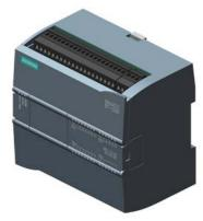
SIMATIC S7-1200, CPU 1214C, compact CPU, DC/DC/DC, onboard I/O: 14 DI 24 V DC; 10 DO 24 V DC; 2 AI 0-10 V DC, Power supply: DC 20.4-28.8V DC, Program/data memory 100 KB
