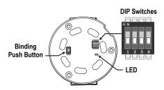
**DIP Switch 1: Radio Transmit Power**—The 900 MHz radios transmit at 1 Watt (30 dBm) or 250 mW (24 dBm). While the Performance radios operate in 1 Watt mode, they cannot communicate with the older 150 mW radios. To communicate with 150 mW radios, operate this radio in 250 mW mode. For 2.4 GHz models, this DIP switch is disabled. The transmit power for 2.4 GHz is fixed at about 65 mW EIRP (18 dBm), making the 2.4 GHz Performance models automatically compatible with older 2.4 GHz models.
