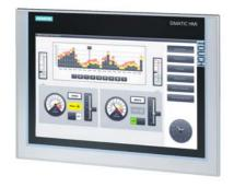
SIMATIC HMI TP1200 Comfort, Comfort Panel, Touch operation, 12" widescreen TFT display, 16 million colors, PROFINET interface, MPI/PROFIBUS DP interface, 12 MB configuration memory, Windows CE 6.0 (Microsoft Support included Security updates discontinued) configurable from WinCC Comfort V11
