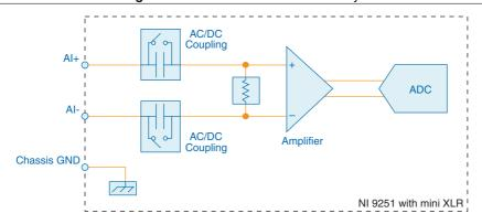
Figure 1. NI 9251 with mini XLR Circuitry
