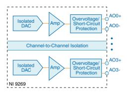
The analog output channels are floating with respect to earth ground and each other. Each channel has a digital-to-analog converter (DAC) that produces a voltage signal. Each channel provides an independent signal path, enabling you to update all four channels simultaneously. Each channel also has overvoltage and short-circuit protection.
